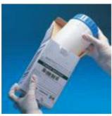
Place the secondary container into the external cardboard carton, and place the sample transfer form between secondary container and the external carton
